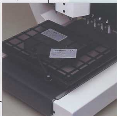
Morsa per tavola scanalata Parallel vise to be used with T-slot worktables
